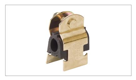
Get a grip – CUSHION CLAMPS are the industry-established method of supporting copper refrigerant tube, especially for multiple pipe runs. The zinc dichromate plating provides excellent corrosion resistance and the polymer insert ensures a positive grip, absorbs shock and vibration and prevents galvanic corrosion.
